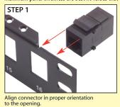
and snap connector in place. Seat Pivot connector upward retainer
