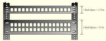
Racks are a great way to neaten up wiring closets and labs. Network equipment and rack panels usually come in 1.75", 3.5" and 5.25" heights. (1, 2 and 3 rack spaces).
